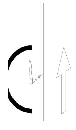
3. Slightly separate the first panel. Move to lead edge and push panel to stack position.
