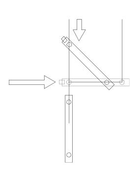
4. Push on face as near the center of the panel possible.
