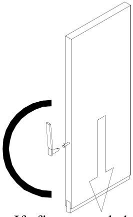
If first panel has flexible vinyl bulb it should be slightly compressed.
