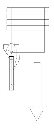
4. While putting slight forward pressure, insert operating handle (pointing up), rotate counter-clockwise approximately 180• until you feel a cam lock action. Lower seals should be down.
