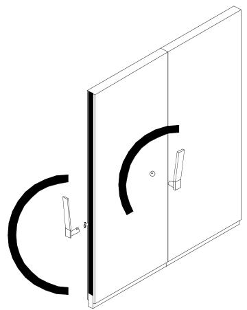
9. Put operating handle into panel face cup and rotate until there is a pronounced cam action.
