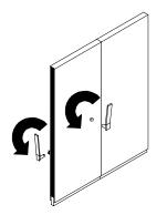
Extend to flat position Insert handle in edge Rotate counterclockwise 180° Insert handle into face receptacle Rotate counterclockwise 180°
